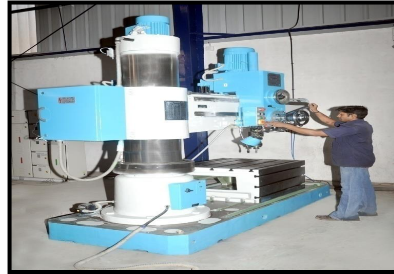
Make: Batliboi Ltd, No. of Qty -3 Size: R1820 mm 360 deg Rot, Vertical-700 mm Max. Drilling capacity: 60 mm
