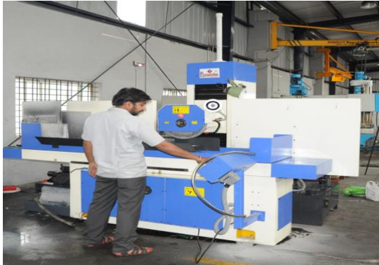
Acer Surface Grinder: No. of 6 Qty Size: 1500 X 600 x 350 mm
