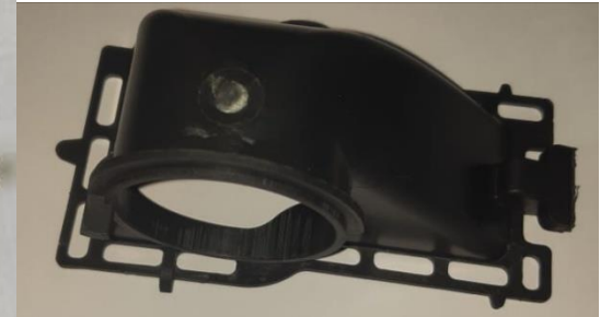
Air Filter Inlet
